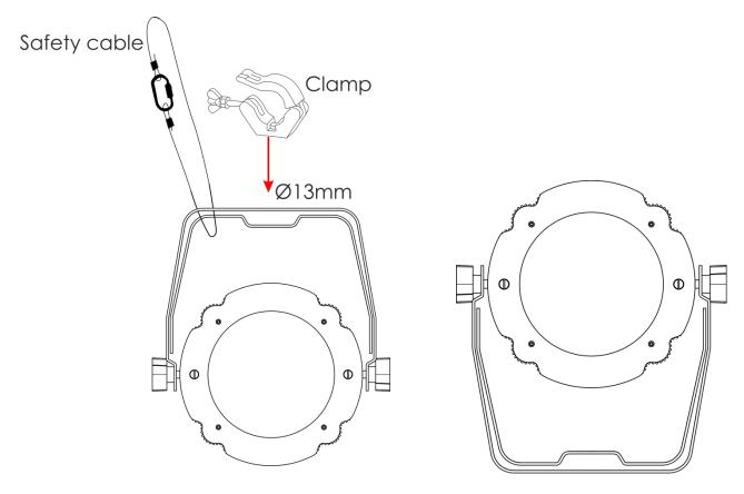
The Compact Par 60 COB RGBW can be placed on a flat stage floor or mounted to any kind of truss with a clamp.
